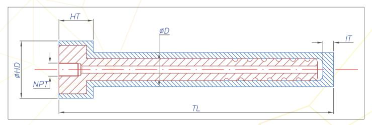
**Cyclone Core™ blanks** are H-13 core pin blanks with internal spiral water line geometry. These can be ordered for finishing by your in-house tool shop, or send us your model if you would like to order with detail completed.
